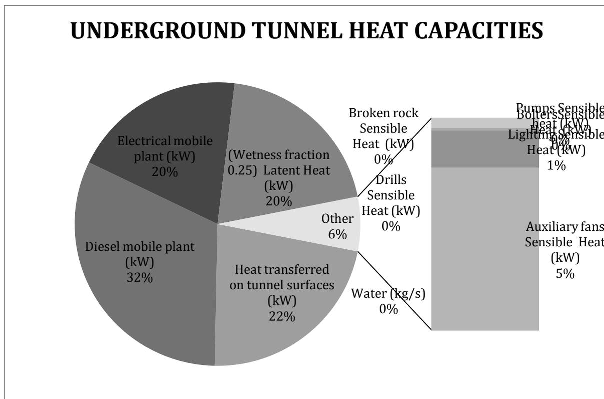
Figure 4: Underground Tunnel Heat Capacities
