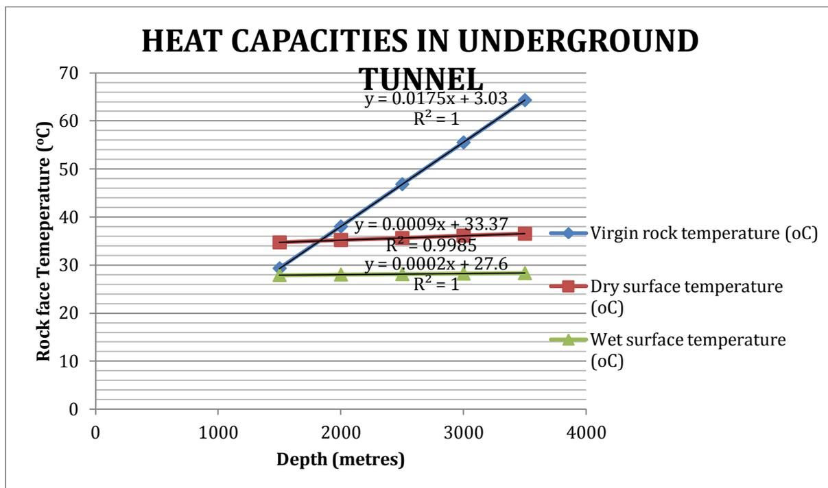
Figure 3: Heat Capacities in Underground Tunnel
