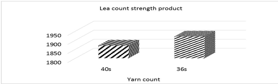
Fig.5. Lea count strength product for ring spun blended yarns at 36s and 40s yarn counts
