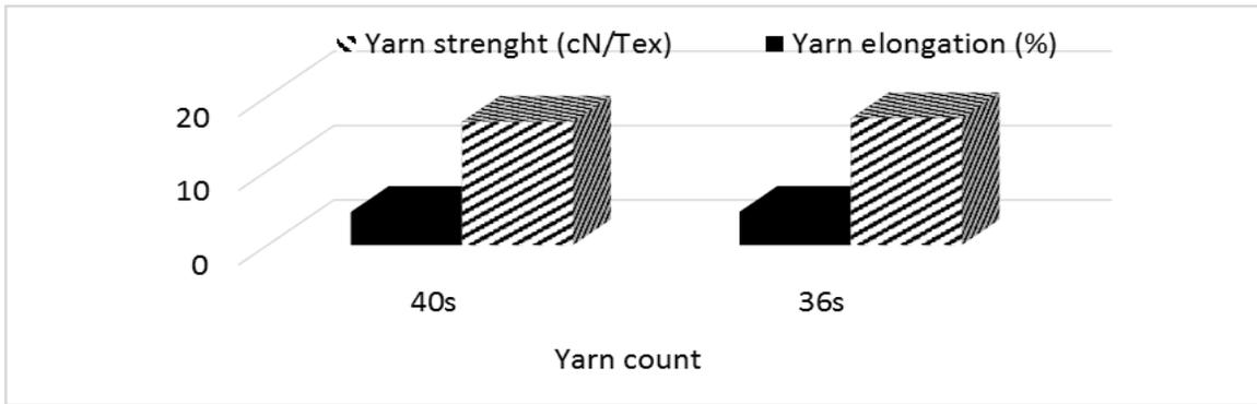
Fig.6. Yarn strength and yarn elongation for ring spun blended yarns at 36s and 40s yarn counts
