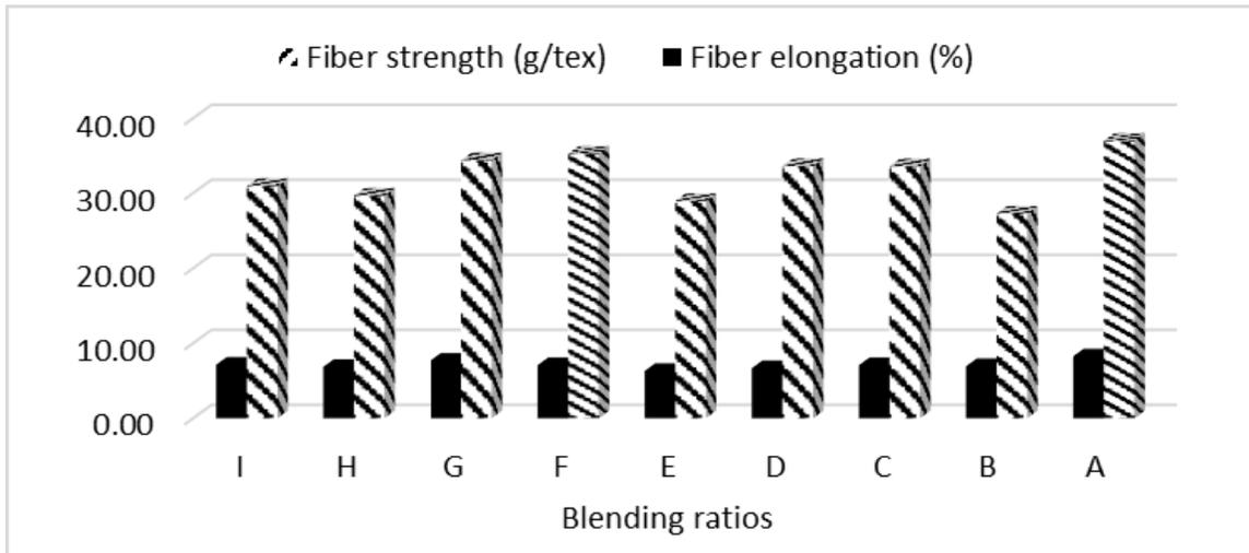
**Fig.2.**Fiber strength (g/tex) and fiber elongation (%) for Giza95, Delta pine 245, combed waste fibers and their blends
