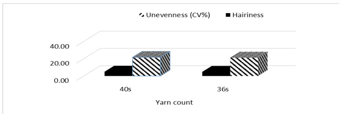
Fig.9. Yarn unevenness (CV %) and yarn hairiness at different yarn counts
