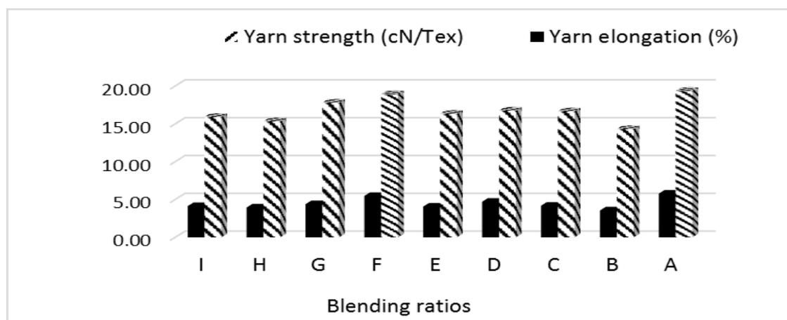
Fig.4. Yarn strength (cN/tex) and yarn elongation (%) of ring spun cotton blended yarns
