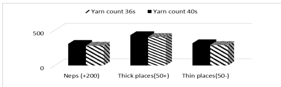
**Fig.8** Number of neps, thin and thick places at different yarn counts
