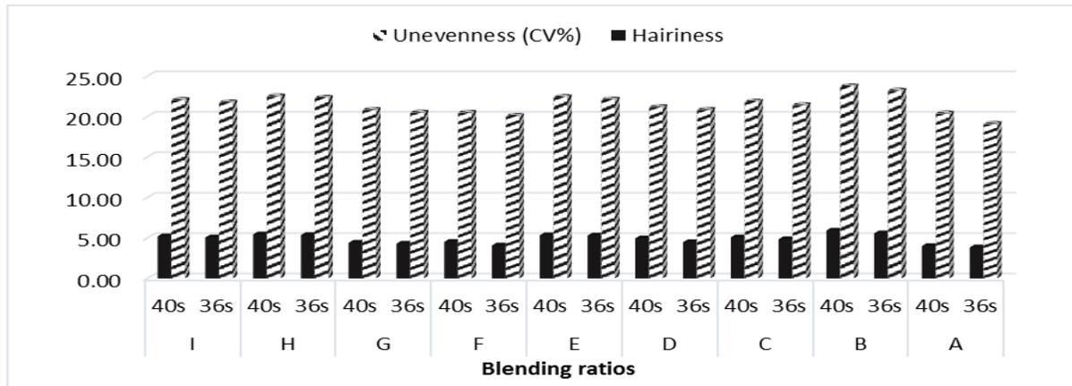
Fig.10. Yarn Unevenness and yarn hairiness for blended yarns at two yarn counts
