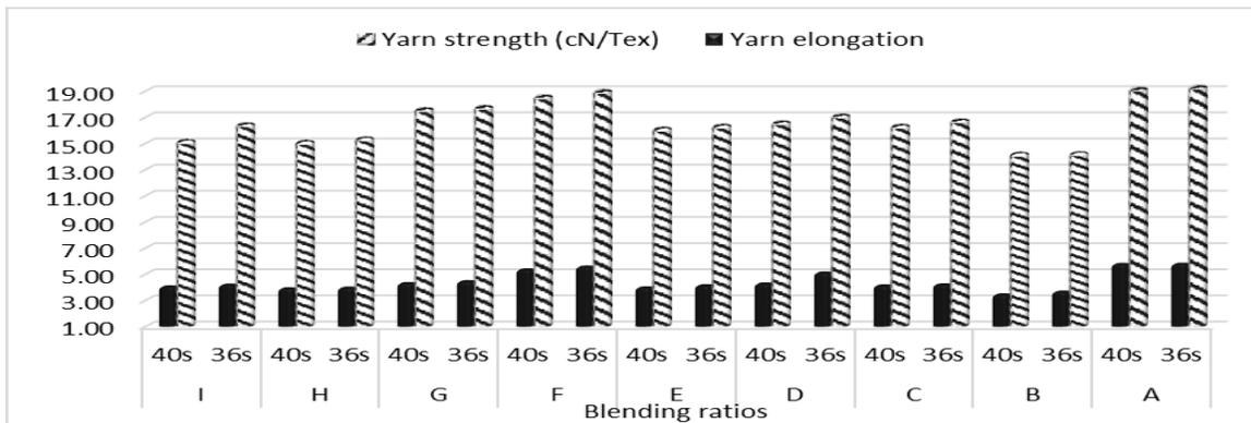
Fig.7. Yarn strength (cN/tex) and yarn elongation (%) for ring spun blended yarns at different yarn counts
