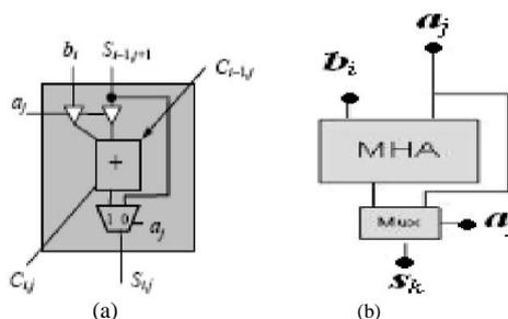
Figure 7: (a) Modified FA cell for column bypassing multiplier. (b) Modified HA cell for column bypassing multiplier.
