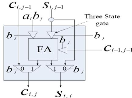
Figure 4. Row Bypassing Adder Cell (RA)
