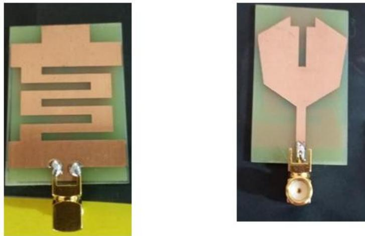
**Fig 10:** Fabricated Front and Rear view of Antenna
