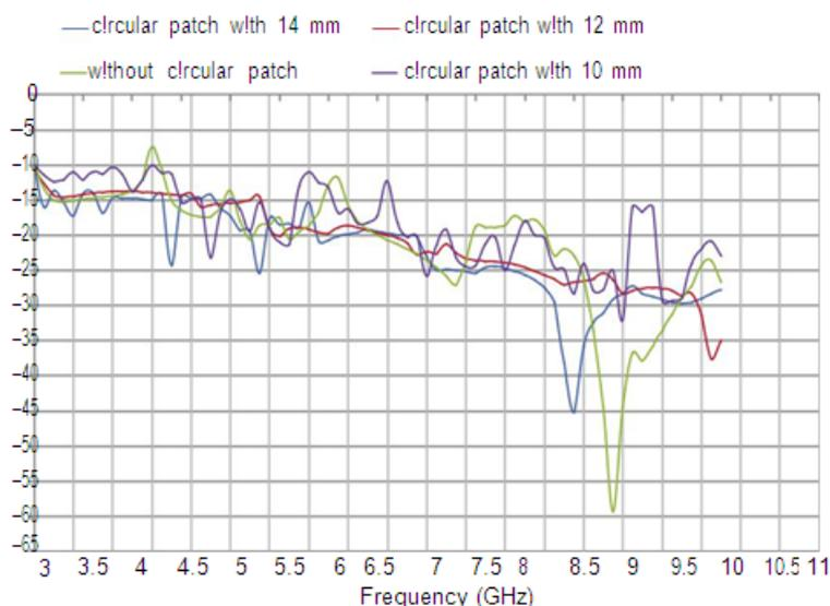
**Figure 7.** Simulated reflection coefficient versus frequency with different values of circular patch.
