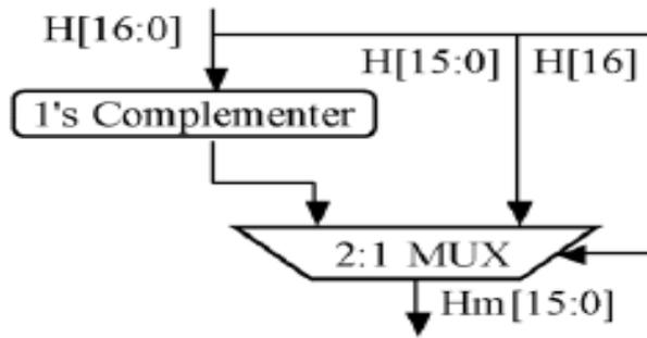
Fig2: Hardware architecture of the Sign Conversion Block.
