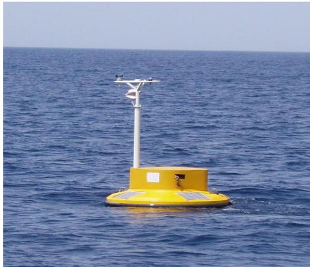
Fig 2: Ambient Noise Buoy
