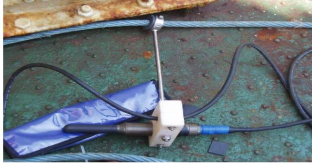
Fig 1: Hydrophone with fixture
