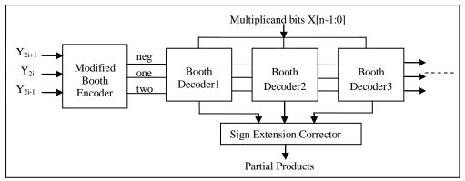
Fig. 5: Structure for generating the partial products.
