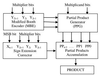
Fig. 1: Block Diagram of Modified Booth Multiplier.
