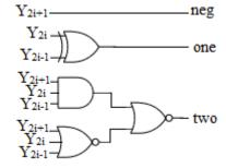
Fig. 4a: Proposed Modified Booth Encoder.
