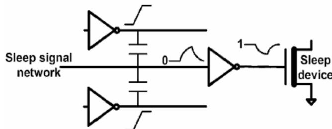
Figure 4: Sleep signal crosstalk noise during active mode.
