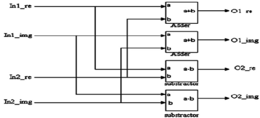
Figure 9: Model of subsystem radix-2\_0
