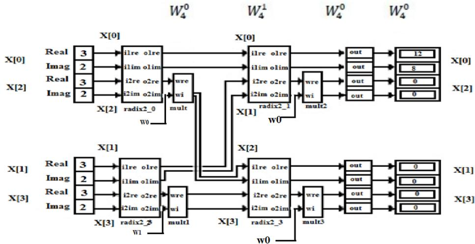
Figure 11: Design of 4 points FFT circuit for parallel input
