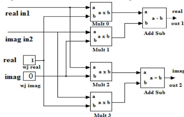
Figure 10: Architecture of the MULTIPLIER subsystem
