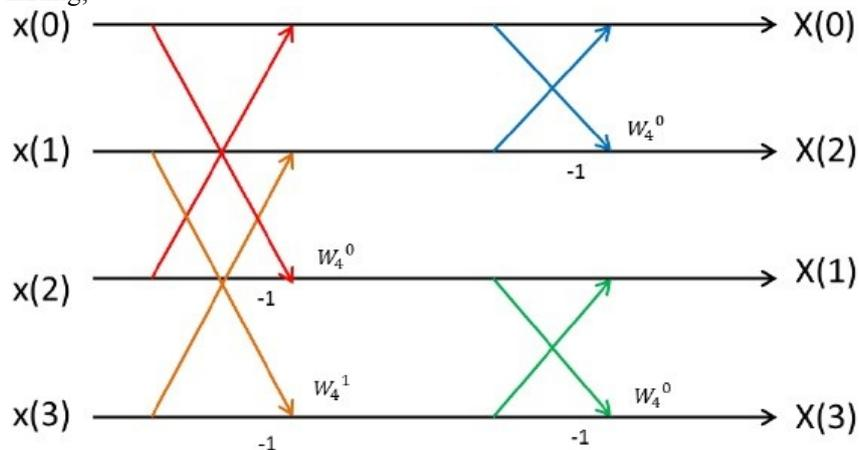
Figure 7: Basic concept of 4-point FFT
