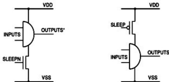
Figure 2: Fine Grain cells
