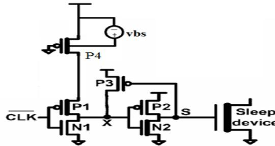
Figure 6: Self sleep buffer using body bias
