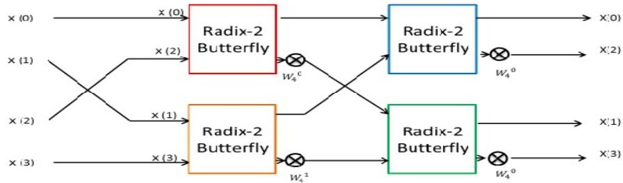
Figure 8: 4 points FFT circuit block diagram
