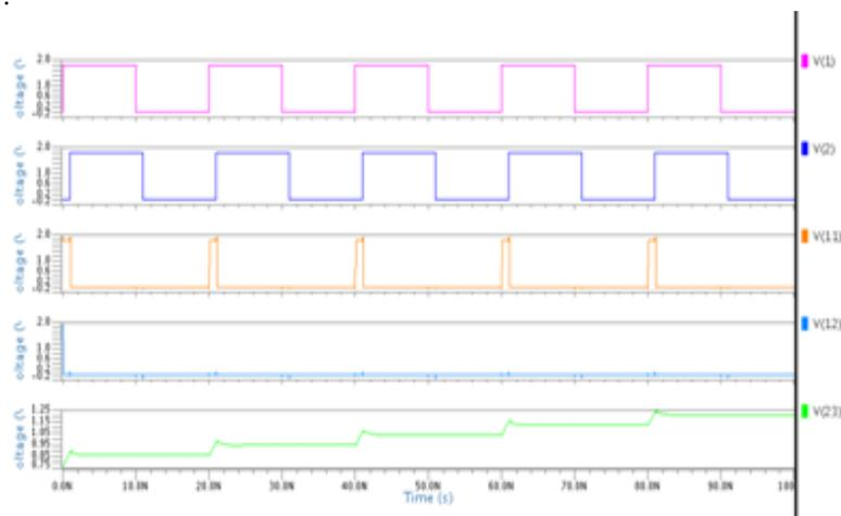
Fig. 7 simulation from phase frequency detector to loop filter at 50MHz
