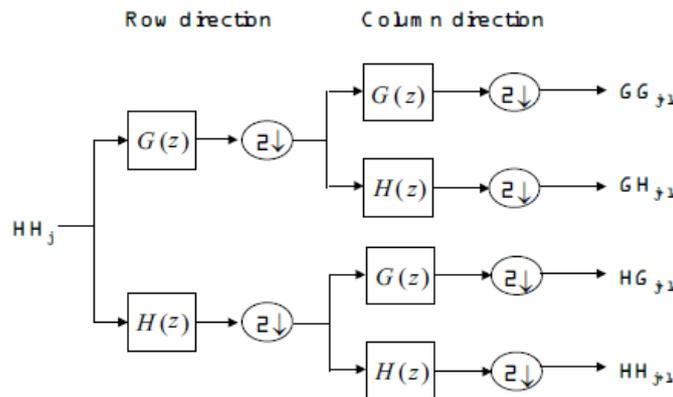
Figure: 6 One level of 8x8 2D DWT (Analysis stage)
