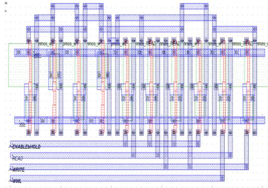
Figure 5: Layout Design of 8T-SRAM
