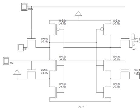
Figure 2: ST1 Bit Cell
