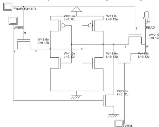
Figure 4: Read Error Reduced 8T-SRAM Cell with Reduced Transistor Count
