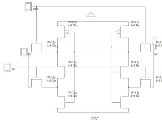
Figure 1: ST2 Bit Cell
