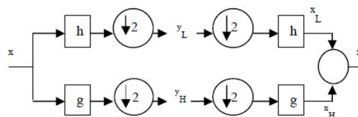
Fig.1 DWT analysis and synthesis system
