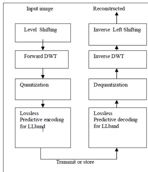
Fig. 4 The block diagram of encoder and decoder.
