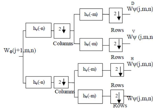
Fig. 2 The 2-D DWT analysis filter bank
