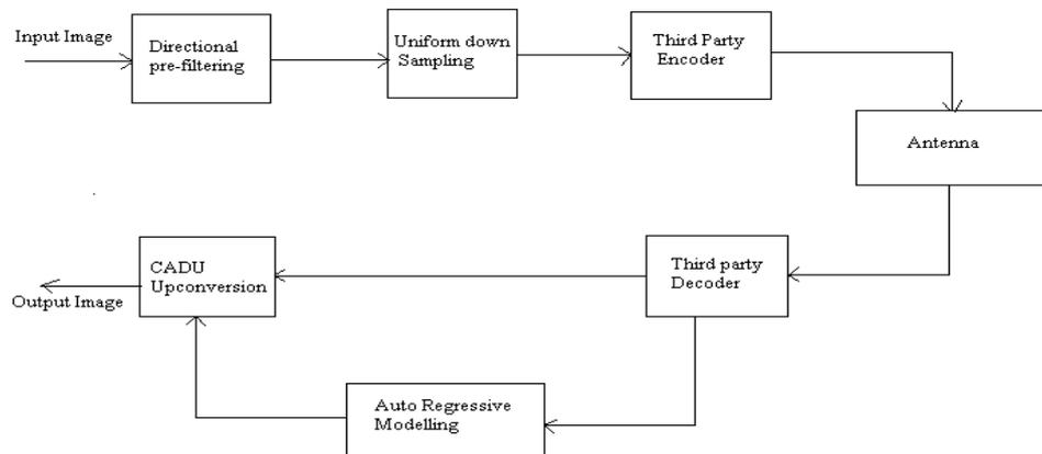
Fig 3. Block Diagram of The Proposed CADU Image Compression System
