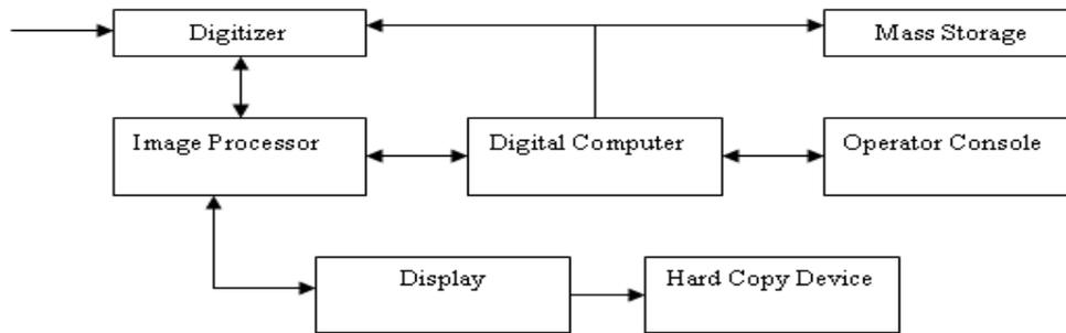
Fig 1. Block Diagram of a Typical Image Processing System
