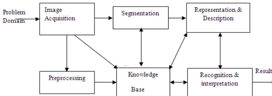
Fig 2. Block Diagram of Fundamental Sequence involved in an image Processing system
