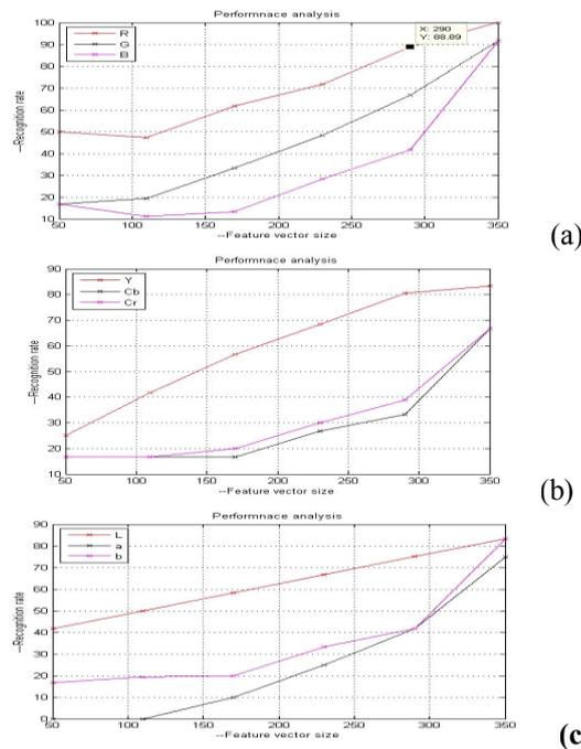
**Fig12:** Comparative evaluation of performance in different color spaces from 128×128 (a)RGB . (b) YCbCr, (c)CIElab
