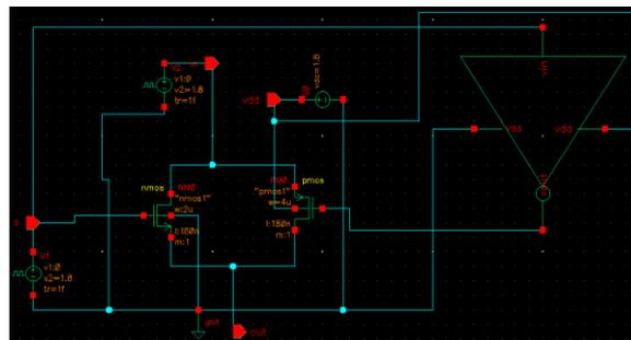
Fig.(w) Schematic of transmission gate
