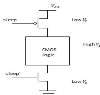
Fig.(f) MTCMOS circuit
