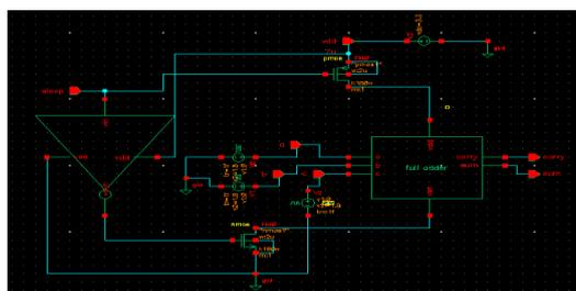
Fig.(g) Schematic View of MTCMOS Circuit
