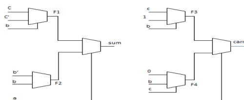
Fig.(d).28T adder circuit using shannon's expansion
