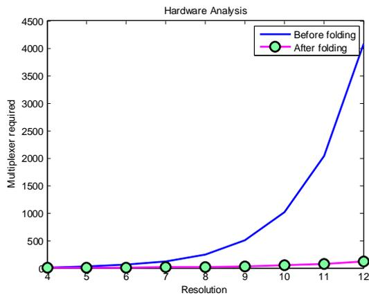
Figure 13: Comparison of Hardware Cost
