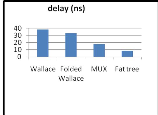
Figure 5 : Propagation delay
