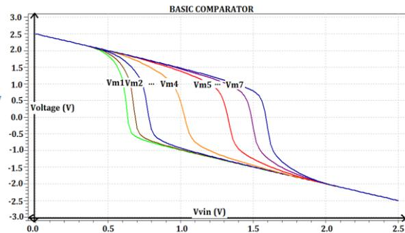
Figure 8: Transfer characteristics of Design I
