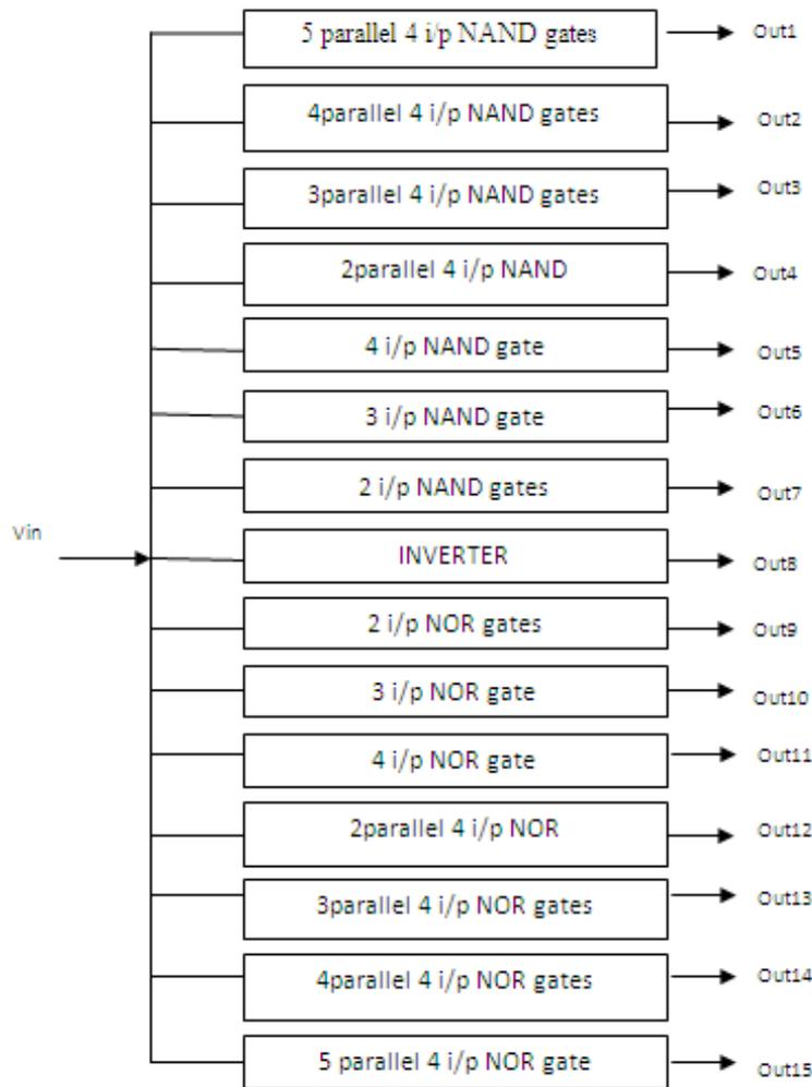
**Figure 1: Design I comparator structure for 4 bit ADC**
