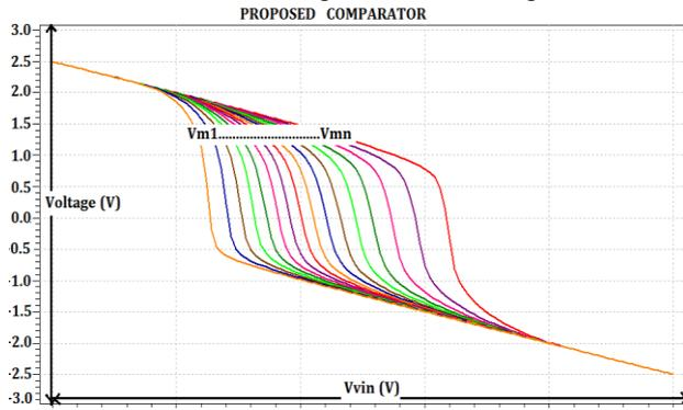
Figure 11: Reference Voltage Selection of Comparator
