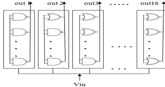
Figure 2: NAND NOR Cell comparator [14]
