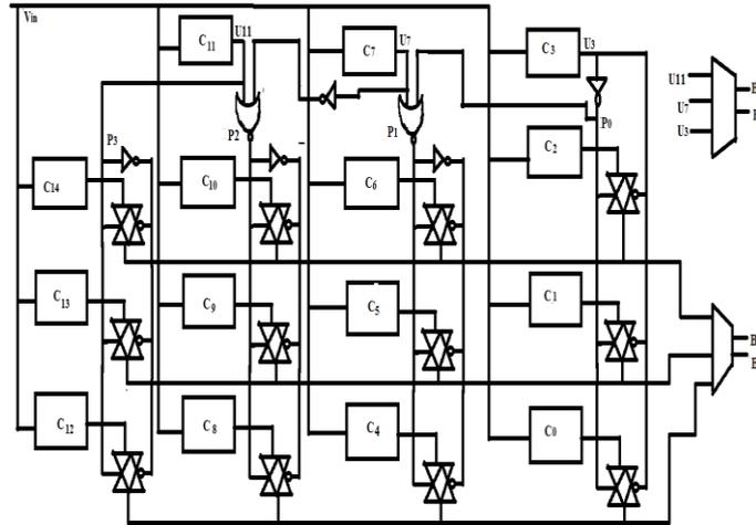
Figure 3: Design of Flash ADC using algebraic partitioning
