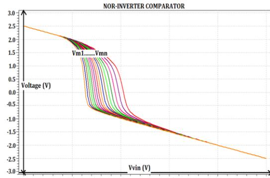
Figure 10: Transfer Characteristics of Design II
