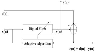
Fig2: Block diagram of Adaptive Filter [4].
