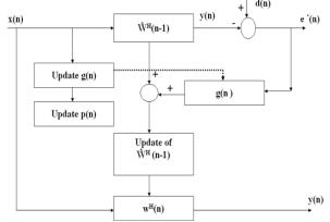
Fig4: Block diagram of RLS Algorithm [13].
