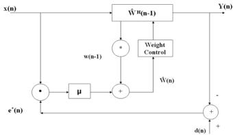
Fig3: Block diagram of LMS Algorithm [13].
