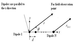
Fig1: Block diagram of linear array [2].
