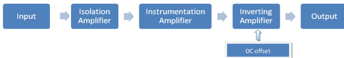
Figure 1: EEG Acquisition System
