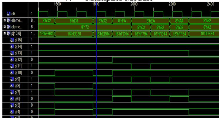
Fig Timing simulation of multiplier unit.
