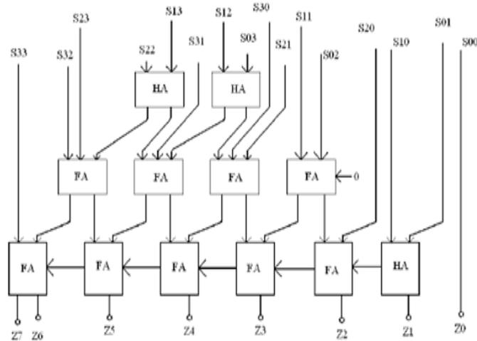
Fig.2 Architecture of a 4x4 Wallace multiplier
