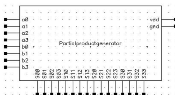
Fig.4 Cellview of partial product generator module
