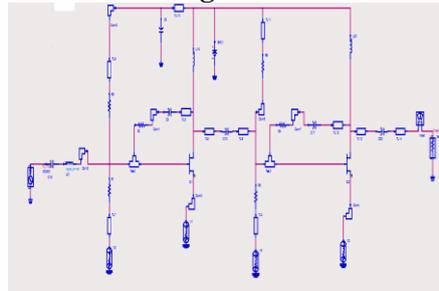
**Figure 3.** ADS schematic for 0.5GHz To 6 GHz UWB Low noise Amplifier
