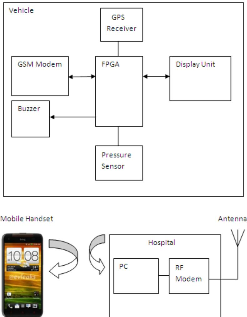
Figure 1. Block diagram for vehicle security and accident information system
