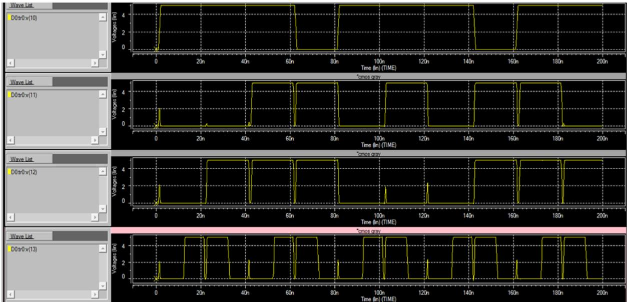
Fig 7: Simulated waveforms for output gray code in DPTL logic.
