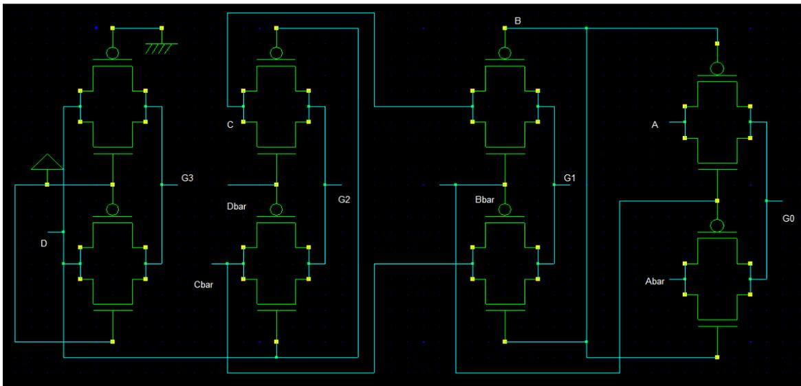
Fig 2: Binary to Gray code converter using DPTL technique
