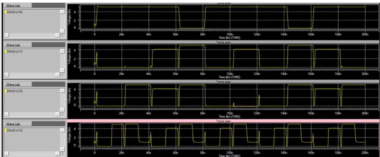
Fig 8: Simulated waveforms for output gray code using 2x1 mux
