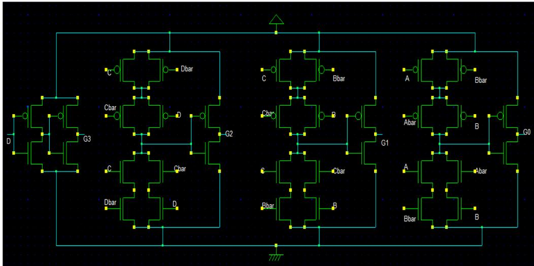
Fig 1: CMOS Binary to Gray code converter
