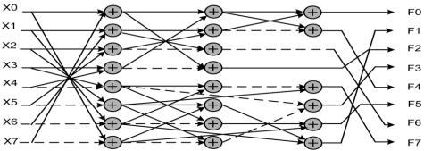
**Fig. 1** Signal flow graph of  $\hat{C}_8$ . Dashed arrows represent multiplications by -1
