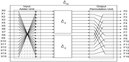
**Fig. 2** Block diagram of the proposed DCT for N = 16 ( $\hat{C}_{16}$ )
