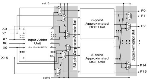
Fig. 4 Proposed reconfigurable architecture for approximate DCT of lengths N = 8, 16 and 32.
