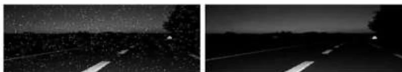
Fig 11: Image with impulse noise (Left) With Median Filter (Right)
