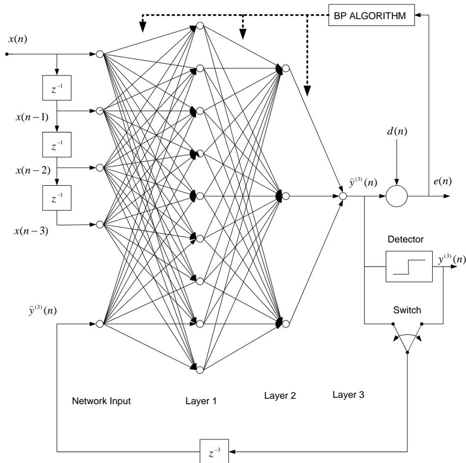
Figure 1: MLP structure for channel equalization
