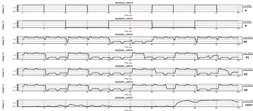
Fig.11. Simulation Waveform of MQSERL Arithmetic Unit
