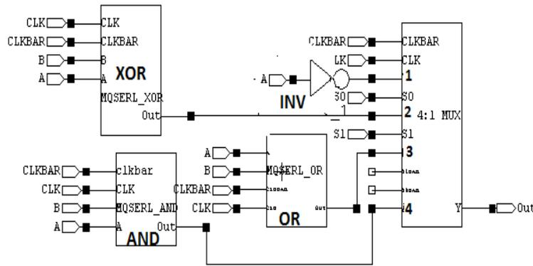
Fig.8. Design of MQSERL LOGIC UNIT
