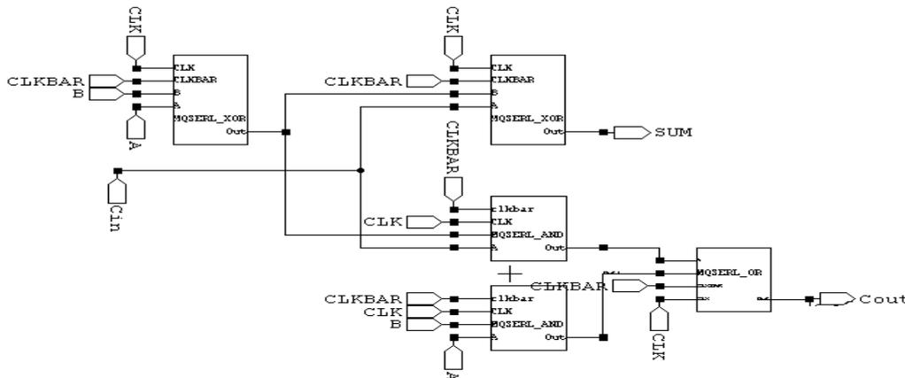
Fig.4.Design of MQSERL Full Adder
