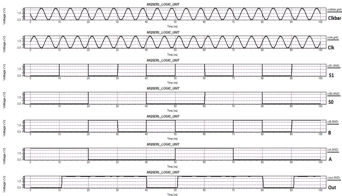
Fig.9.Simulation Waveform for MQSERL LOGIC UNIT
