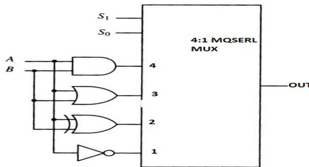
Fig.7.Design of Logic Unit
