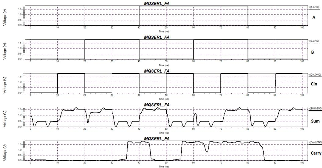
Fig. 5 Simulation Waveform of MQSERL FULL ADDER
