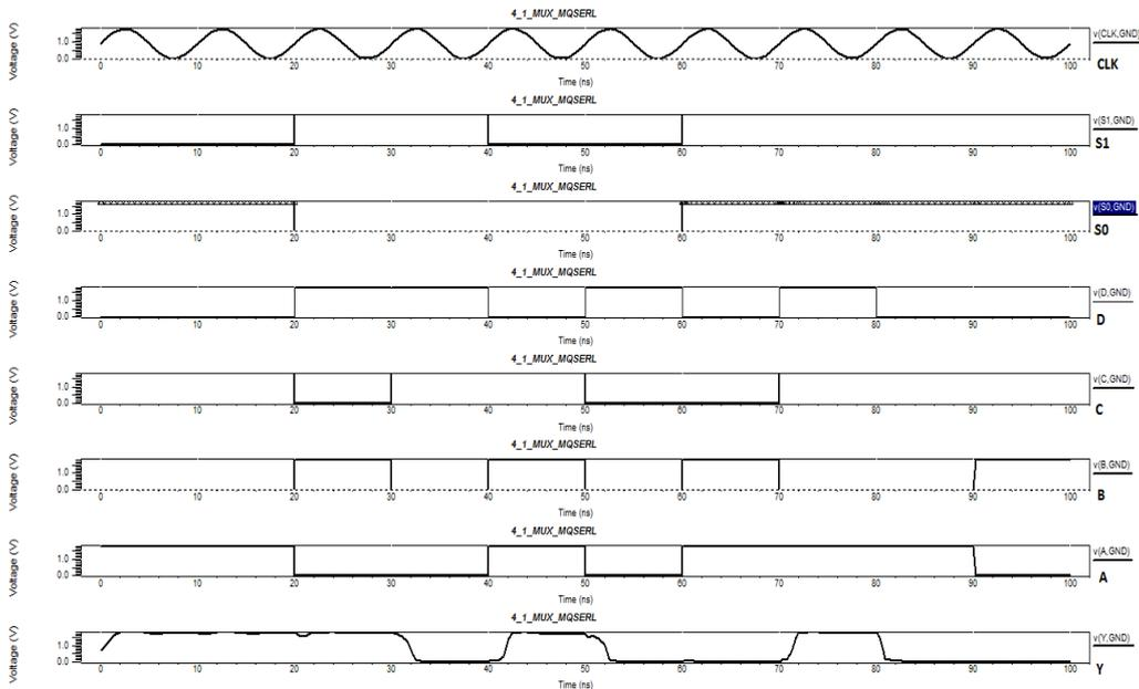
Fig.3.Simulation Waveform of 4:1 MQSERL MUX
