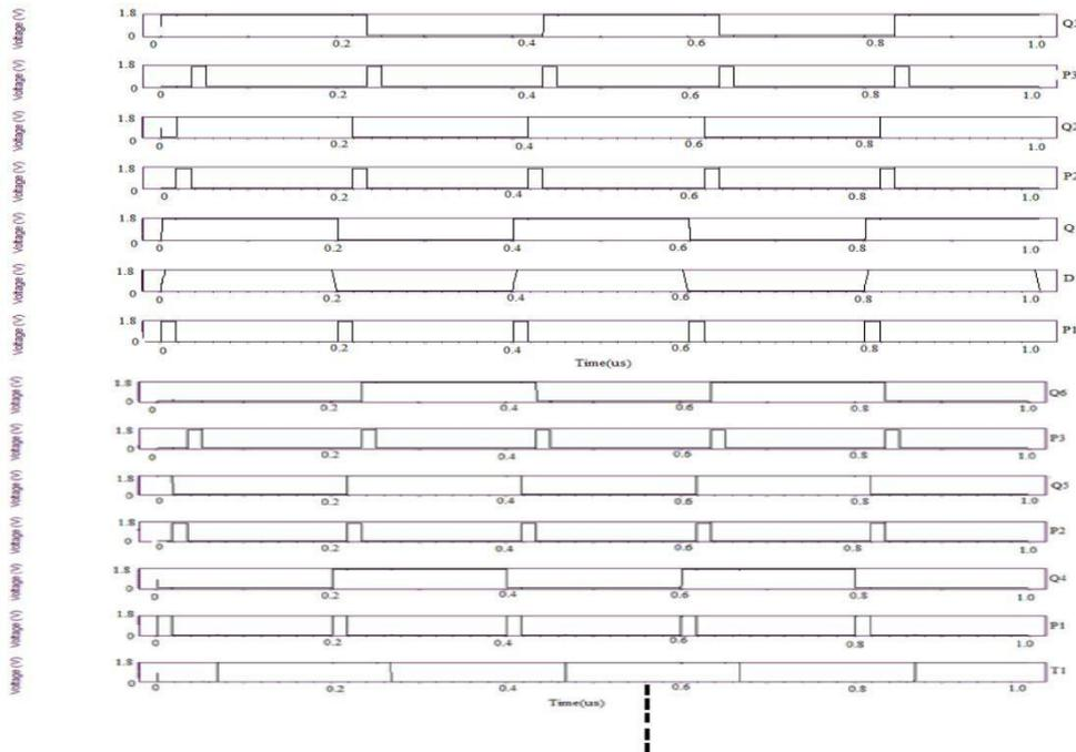
**Fig.12** Simulated waveforms of 512-bit SSASPL shift register
