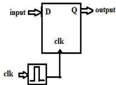
Fig.2 Pulsed latch circuit
