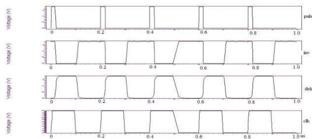
**Fig.7** Simulation result of Pulse Generation circuit
