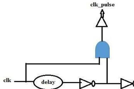
**Fig.6** Pulse Generation Circuit
