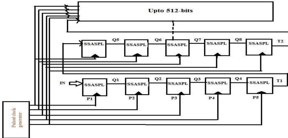
**Fig.11** 512-bit SSASPL shift register
