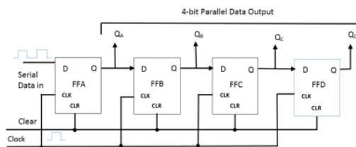
Figure 2: Circuit diagram of SIPO shift register
