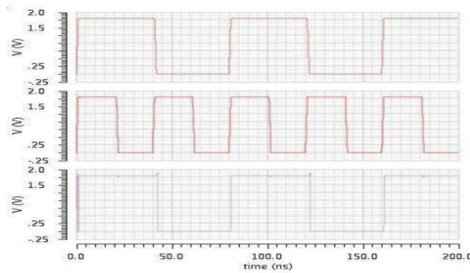
Figure 12: Simulation Design Implementation of SISO shift register
