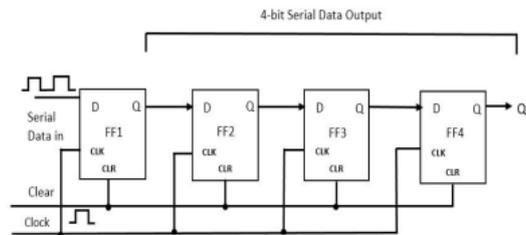
Figure 1: Circuit diagram of SISO shift register
