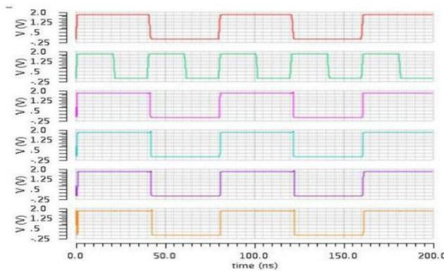
Figure 13: Simulation Design Implementation of SIPO shift register
