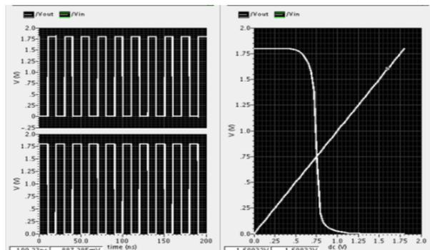
Figure 9: Simulation Design Implementation of Inverter
