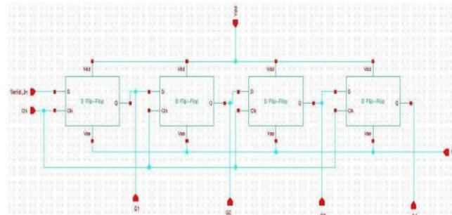
Figure 8: Schematic design implementation of SIPO shift register
