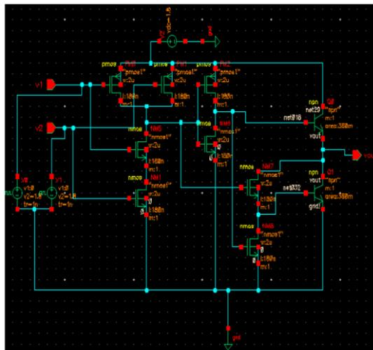
Figure 5: Schematic design implementation of AND gate
