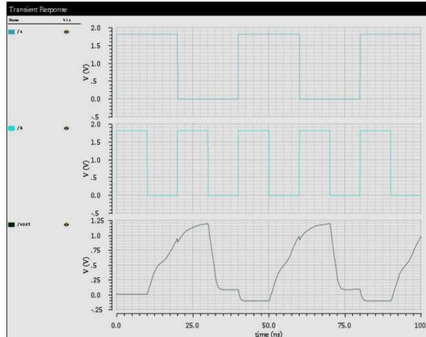
Figure 11: Simulation Design Implementation of XOR gate
