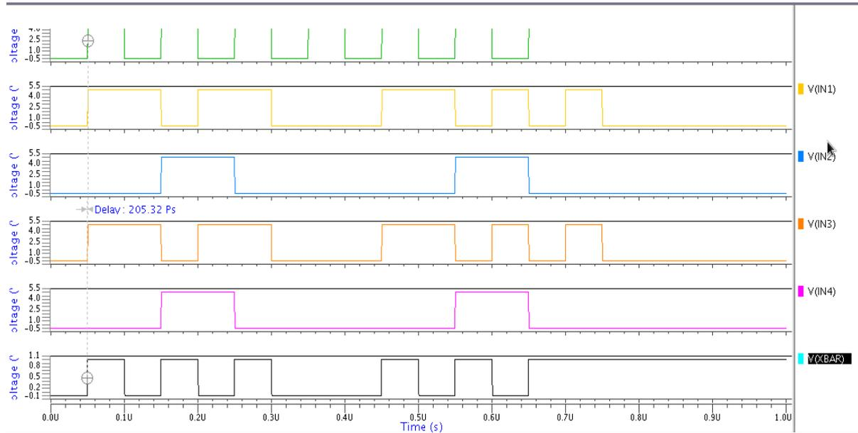
Fig 20. Waveforms of Comparator based domino logic for wide fan-in OR gate
