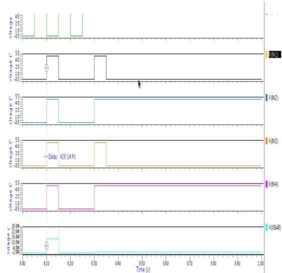
Fig. 9. Waveforms of High Speed Clocked Delay Domino Logic
