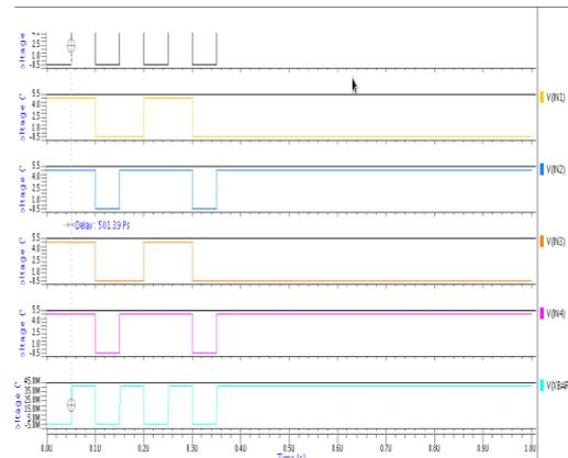
Fig. 7. Waveforms of Current Mirror Footed Domino Logic
