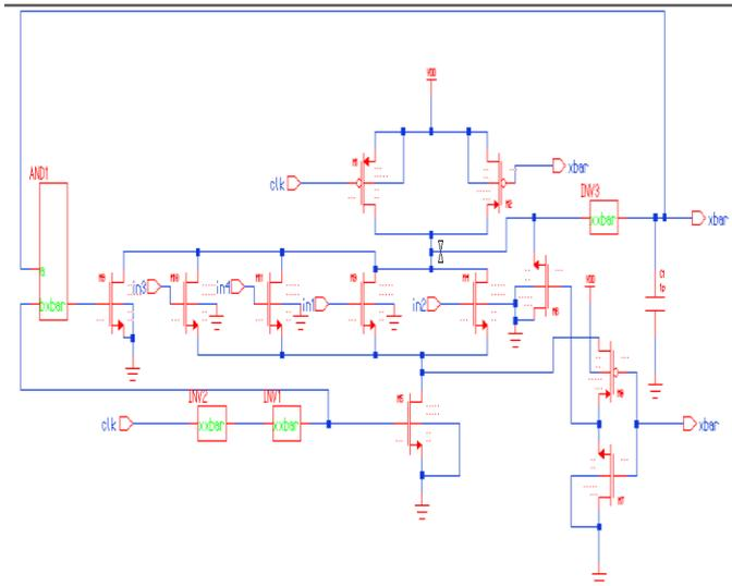
Fig. 11. Modified High Speed Clocked Delay Domino Logic
