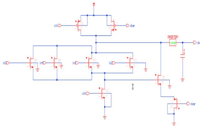
**Fig. 17** Foot Driven Stack Transistor Domino Logic
