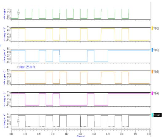
**Fig. 18** Waveforms of Foot Driven Stack Transistor Domino Logic
