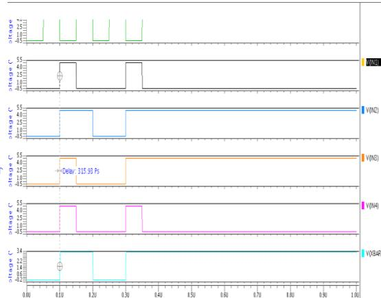
**Fig. 2** Waveforms of Footerless Domino Logic
