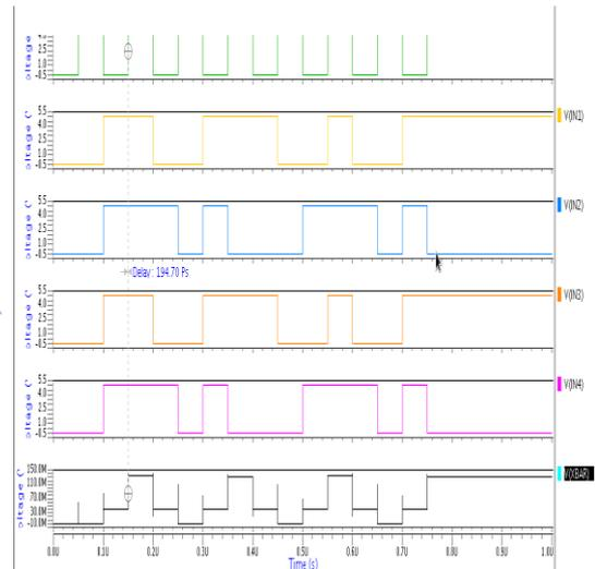
**Fig. 16** Waveforms of Conditional Stacked Keeper Domino logic
