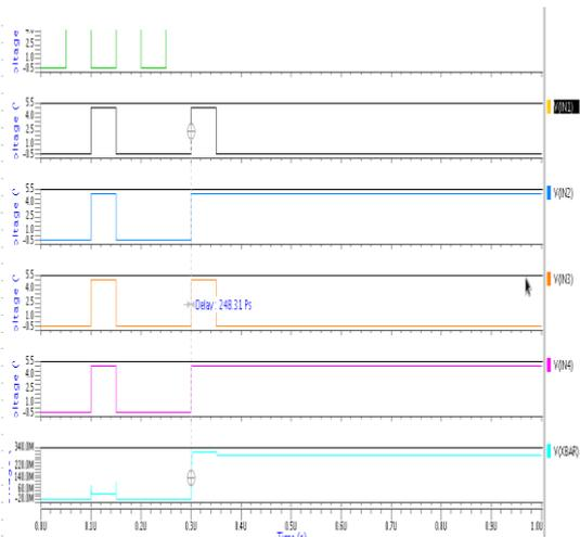
Fig.14. Waveforms of Conditional Evaluated Domino Logic
