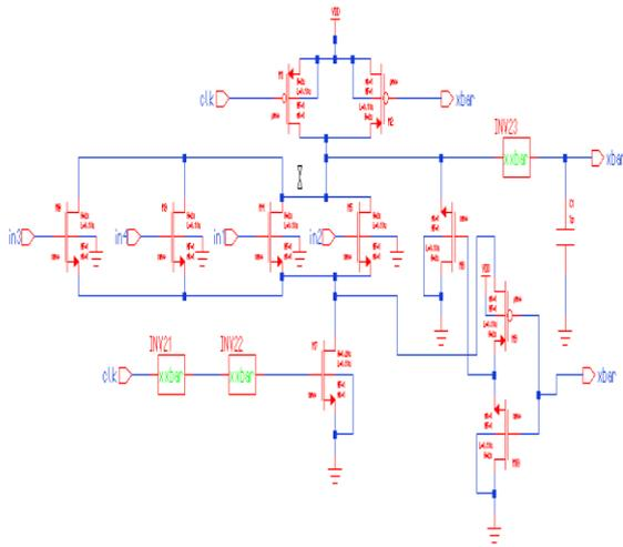
Fig. 8. High Speed Clocked Delay Domino Logic
